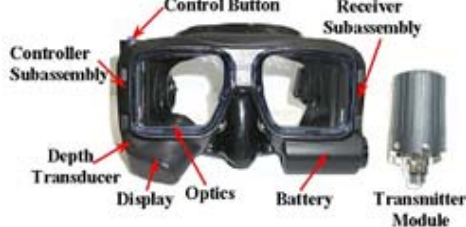
IDDM System components.
